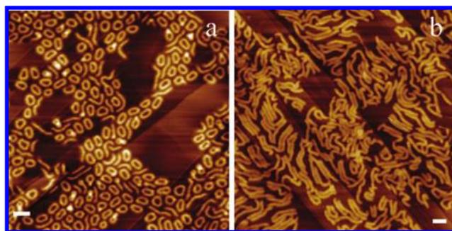
**Figure 7.** AFM image of cyclic combs after treatment in acidic media.
